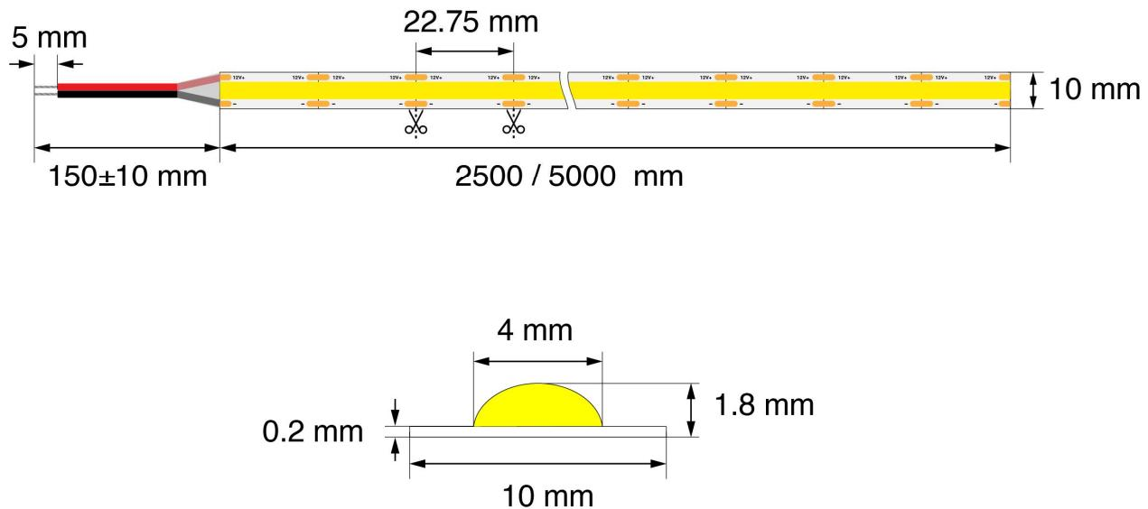
The LED strips can be easily separated or shortened at the intersection using the cutter. There is double-sided heat-conducting adhesive tape on the back of the LED strips, which makes installation quick and easy.
