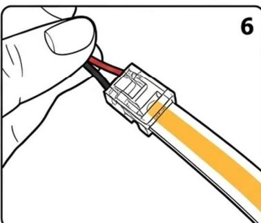
The original LED strip has a cable connection on one side. After shortening the LED strips, a new connection can be made through a connector provided for this purpose.
