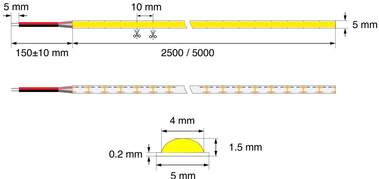
The LED strips can be easily cut to length at the designated cutting points. Each strip features a double-sided, thermally conductive adhesive tape on the back, allowing for quick and simple installation
