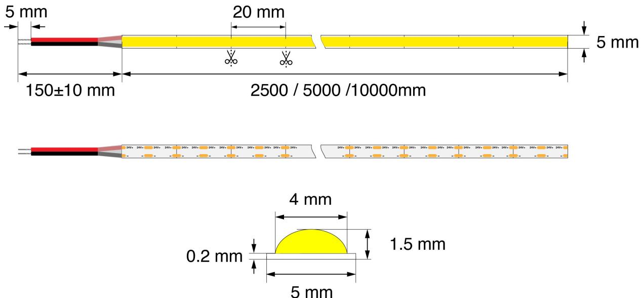
The LED strips can be easily separated or shortened at the intersection using the cutter. There is double-sided heat-conducting adhesive tape on the back of the LED strips, which makes installation quick and easy.
