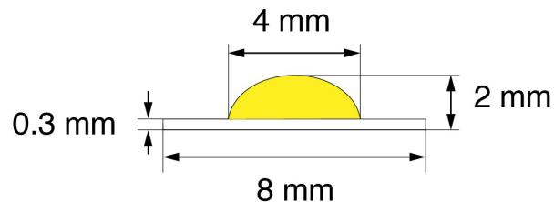
The LED strips can be easily separated or shortened at the intersection using the cutter. There is double-sided heat-conducting adhesive tape on the back of the LED strips, which makes installation quick and easy.
