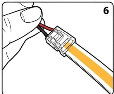
The original LED strip has a cable connection on one side. After shortening the LED strips, a new connection can be made through a connector provided for this purpose.
