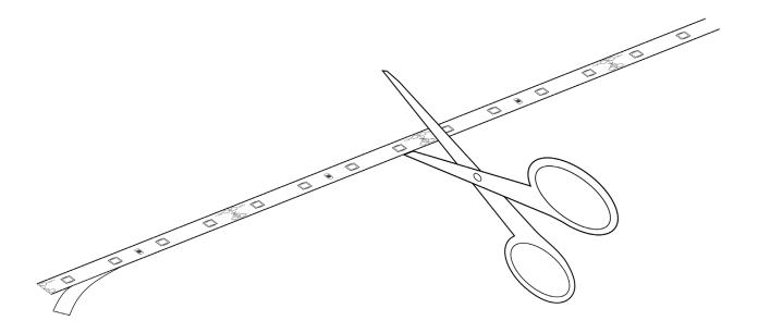
The LED strips can easily be separated or shortened with a cutter at the point of intersection. There is a double-sided, thermally conductive adhesive tape on the back of the LED strips, which enables the LED strips to be installed quickly and easily.
