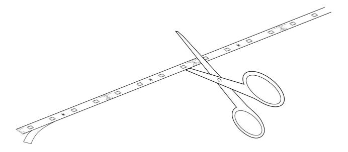
The LED strips can easily be separated or shortened with a cutter at the point of intersection. There is a double-sided, thermally conductive adhesive tape on the back of the LED strips, which enables the LED strips to be installed quickly and easily.
