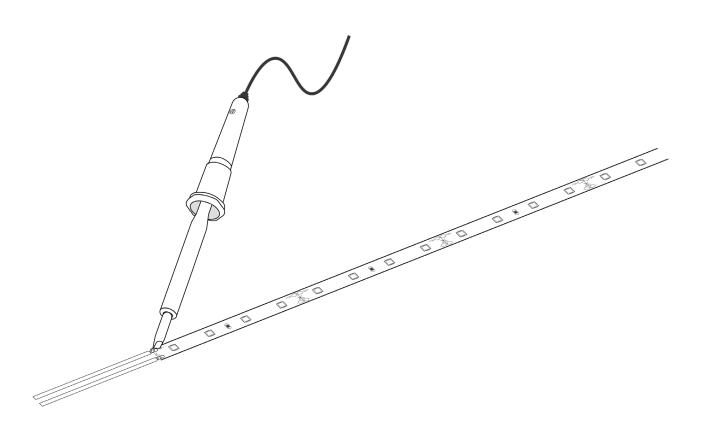
The original 5m LED strip has a cable connection on one side. After shortening the LED strips, a new connection can be made through soldering cable on the soldering pads provided for this purpose.
