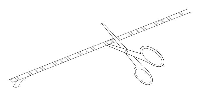
The LED strips can easily be separated or shortened with a cutter at the point of intersection. There is a double-sided, thermally conductive adhesive tape on the back of the LED strips, which enables the LED strips to be installed quickly and easily.
