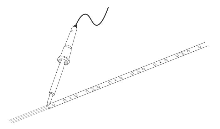
The original 5m LED strip has a cable connection on one side. After shortening the LED strips, a new connection can be made through soldering cable on the soldering pads provided for this purpose.
