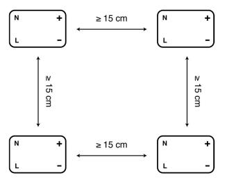
Make sure there is a clearance of at least **15cm** between the LED driver and other heat sources, e.g., other LED power supplies, lamps/LEDs etc.
