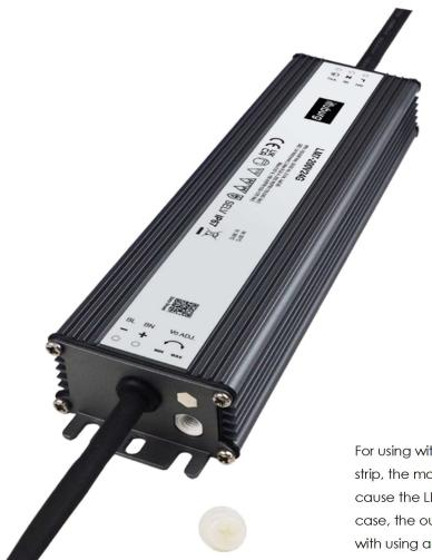
For using with long LED strips, the longer the LED strip, the more loss of output voltage. This may cause the LED strip to darken or flicker. In this case, the output voltage can be adjusted +/-10% with using adjusting screw on the housing.
