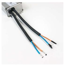
If only single output is used. The unneeded output cable should be insulated with cable terminal or electrical tape.
