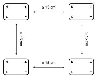
Make sure there is a clearance of at least **15cm** between the LED driver and other heat sources, e.g., other LED power supplies, lamps/LEDs etc.
