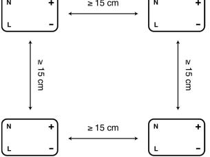
Make sure there is a clearance of at least **15cm** between the LED driver and other heat sources, e.g., other LED power supplies, lamps/LEDs etc.
